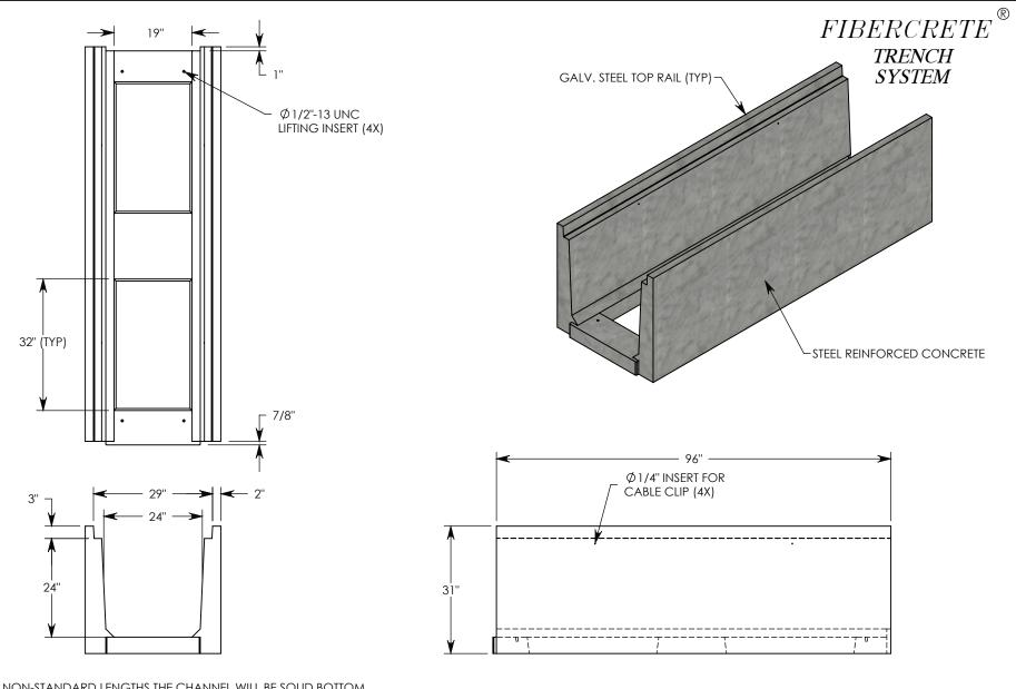
NOTE: FOR NON-STANDARD LENGTHS THE CHANNEL WILL BE SOLID BOTTOM AND DESIGNATED WITH ITS CORRESPONDING LENGTH MEASUREMENT. IE:802424LT 32"
