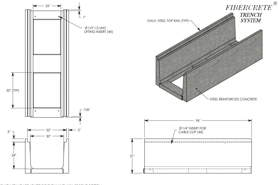
NOTE: FOR NON-STANDARD LENGTHS THE CHANNEL WILL BE SOLID BOTTOM AND DESIGNATED WITH ITS CORRESPONDING LENGTH MEASUREMENT. IE: 803024LT 32"
