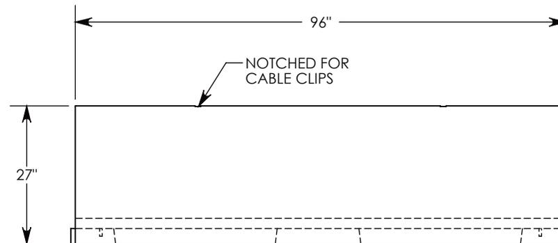
**NOTE:** FOR NON-STANDARD LENGTHS THE CHANNEL WILL BE SOLID BOTTOM AND DESIGNATED WITH ITS CORRESPONDING LENGTH MEASUREMENT. IE: 884024PT 32"
