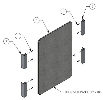
NOTE: DESIGNED TO CREATE SEPARATION IN A 30" WIDE BY 36" TALL CONCAST FHR HANDHOLE UNIT.
