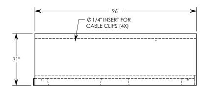
**NOTE 1:** FOR NON-STANDARD LENGTHS THE CHANNEL WILL BE SOLID BOTTOM AND DESIGNATED WITH ITS CORRESPONDING LENGTH MEASUREMENT. IE: LTF1024 36"
