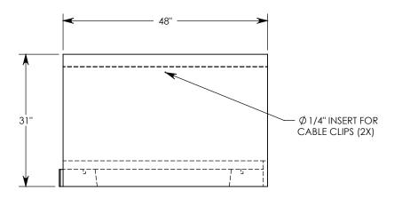
**NOTE 1:** FOR NON-STANDARD LENGTHS THE CHANNEL WILL BE SOLID BOTTOM AND DESIGNATED WITH ITS CORRESPONDING LENGTH MEASUREMENT. IE: LTF3024 36"
