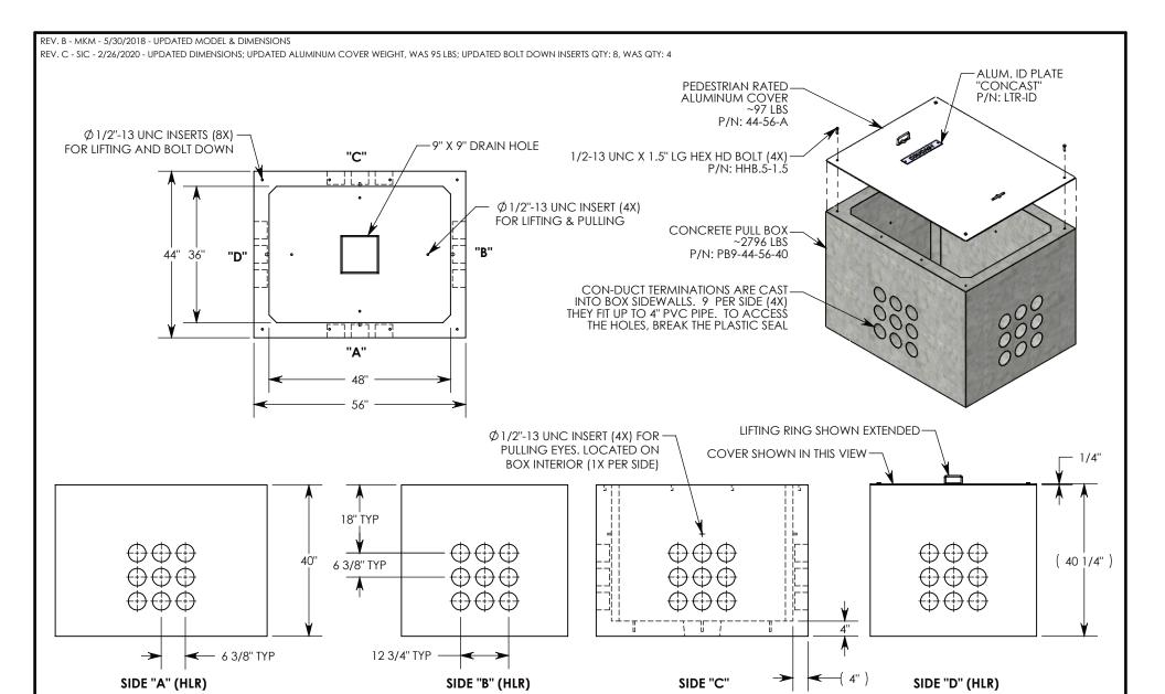
NOTE 1: FOR PVC SIZES SMALLER THAN 4", USE CONCAST RC41 (REDUCING COUPLER) NOTE 2: FOR ADDED SECURITY, PENTA HEAD BOLTS (P/N: PTA.5-1.5) CAN BE ADDED
