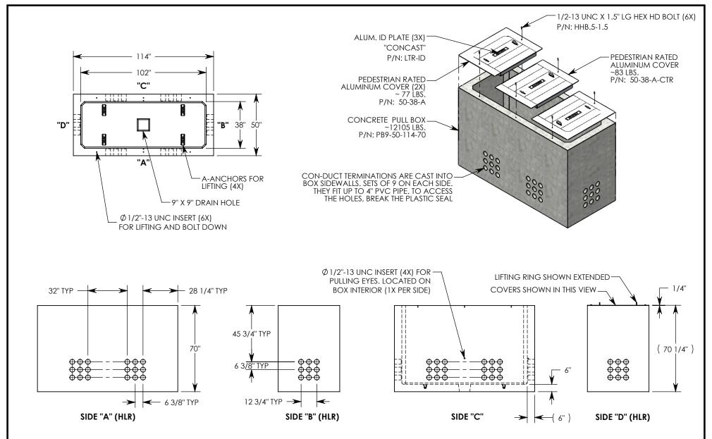
NOTE 1: FOR PVC SIZES SMALLER THAN 4", USE CONCAST RC41 (REDUCING COUPLER).
