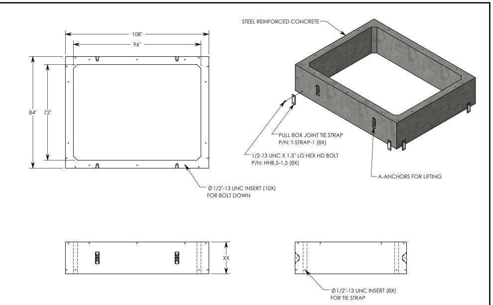
NOTE 1: XX CAN BE ANY HEIGHT, IN 1 INCH INCREMENTS, FROM 12" (MIN) TO 65" (MAX) EX: A 24" EXTENSION WOULD BE NAMED PBEX-84-108-24
